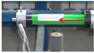
5. Slide the new motor into position & refit the end cap
